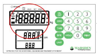
The scale will first test all of the display segments.
