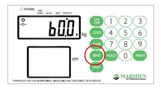
Press the BMI button to return normal mode and the person can now be taken off the scale.
