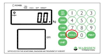
Press HOLD again to unlock the weight and return to 0.0kg
